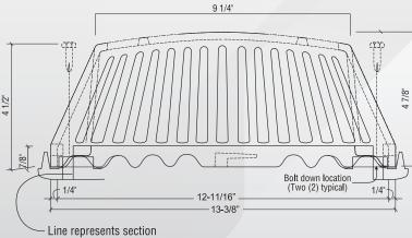
of base ring showing location of 5/16" tapped hole for bolt down of strainer.
