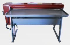
Made to cut material from 30 to 16 gauge with sheet capacity of 48" wide. Three pair of high carbon/high chrome steel knives. Powered by 115 volts 1/3 hp electric motor.
