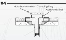
Place Marathon's Aluminum Clamping Ring over metal studs and install supplied stainless steel nuts and washers. Tighten clamping ring against membrane flashing until secure. Do not over tighten as the possibility of the ring or studs could be damaged.
