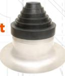
The Uni-Boot provides a permanent watertight and maintenance free means for penetrating roof systems. It is able to be used on all types of roof systems while eliminating the need for pitch pans. Made from EPDM, rubber caps and spun aluminum base, the Uni-Boot eliminates roof leaks from roof penetrations.
