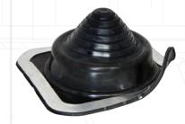
Premium roof flashing that is available in many sizes with a flexible cone, low profile design, bonded aluminum flange and available to be painted to match floor color, EPDM will withstand temperature of -122 F to 392 F for intermittently temperatures. Silicone will withstand constant temperatures of -112 F to 392 F.
