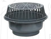
10" or 12" RD-500 Super Flow epoxy coated cast iron roof drain with flashing clamp with integral gravel stop, self-locking ductile iron dome, and no hub outlet.
