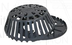
Versatile easy and quick replacement for broken or missing roof drains domes and rings. Maximum drainage, strong cast aluminum and bolt down security. Fits three or four bolt patterns ranging from 6-1/2" to 11-3/4". V channel scallops openings on the ring and dome allow for maximum drainage.
