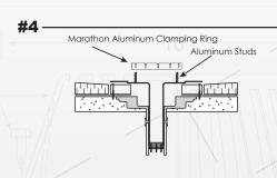
Place Marathon's Aluminum Clamping Ring over metal studs and install supplied stainless steel nuts and washers. Tighten clamping ring against membrane flashing until secure. Do not over tighten as the possibility of the ring or studs could be damaged.
