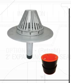
For Use With: All types of roofing materials Job Preparation: Remove existing Strainer and Clamping Ring. Remove any other existing drain components as required to enable our Aluminator Drain flange to lie flush on roof membrane. Remove any debris in the existing drain pipe that interferes with proper installation.
