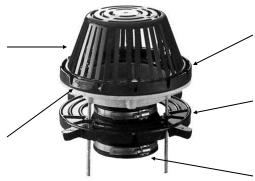
Epoxy Coated aluminum clamping collar with gravel stop. Grooved for positive drainage on smooth surfaced roofs. Distortion resistant and unbreakable. 10" diameter for 2", 3" and 4" sizes. 12" diameter for 6" & 8".
