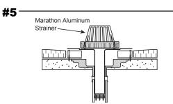
Install Marathon's Aluminum Strainer by aligning screw holes with the holes in the clamping ring. Secure with screws provided.
