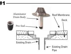
Inspect the existing drain pipe to make sure there are no elbows that prevent the drain stem from being fully inserted into the pipe. If an elbow is present, follow directions on back page to shorten our Aluminator Drain length. Insert Pro-Seal into end of drain stem and tighten screws enough to hold the seal in place during installation. Insert assembled Aluminator Drain into existing drain pipe until flange is flush on roof membrane.
