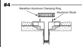
Place Marathon's Aluminum Clamping Ring over metal studs and install supplied stainless steel nuts and washers. Tighten clamping ring against membrane flashing until secure. Do not over tighten as the possibility of the ring or studs could be damaged.
