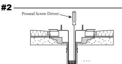
Alternately tighten seal compression ring screws with Pro-Seal Screwdriver until hand tight. Aluminator Drain body is correctly installed when pressure placed on drain body results in no vertical movement. Do not overtighten the screws.
